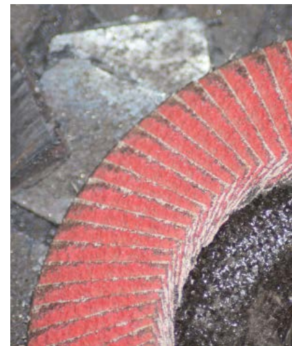
Ceramic material after several minutes of heavy grinding.
